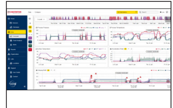
Chesterton Connect data helped solve the seal failure problems.
