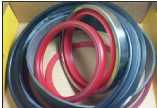
Custom kits developed specifically for the tilt and lift cylinders of the Caterpillar® D11R.
