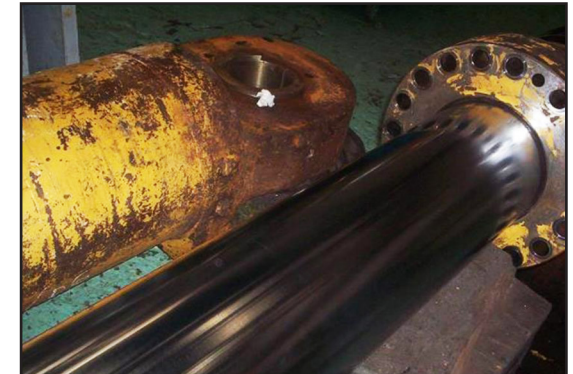
Arm cylinder was in excellent condition upon inspection.
