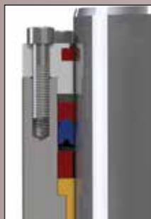
Large stuffing box depth. Backup ring (9K) protects seal (11K) against extrusion while spacer fills up the axial space in front of the seal set.
