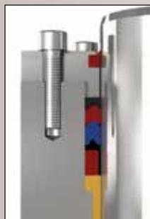
Large stuffing box depth. Customized Self-aligning gland ring provides superior resistance against extrusion in case of large extrusion gap (worn bushings, worn rams).
